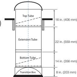
\*Compatible with dome ring to be used as a top tube or extension tube
