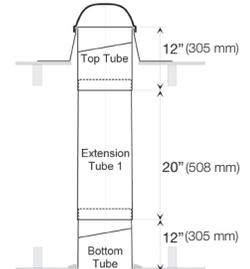
Assuming 6 in. (152 mm) high no-pitch flashing
