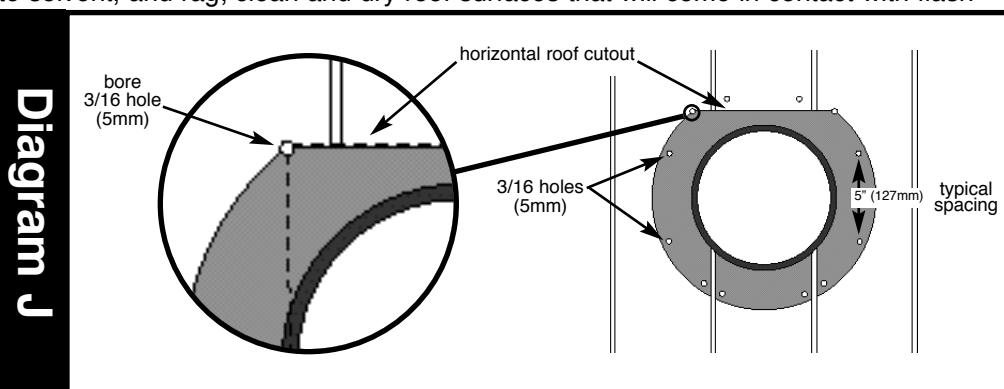
**Step 8.** Apply butyl sealant tape to one side of two corner washers and insert fasteners as shown. Place speed nuts (flat side up) over protruding screw shanks and tighten fasteners to sandwich butyl sealant tape. Then drive flashing screws through flashing and roof panel as shown. Place speed nuts (flat side up) on downside of roof panel, over protruding screw shanks, and tighten fasteners to sandwich butyl sealant tape. Note: Use vicegrips to hold speed nuts. **Diagram K**
