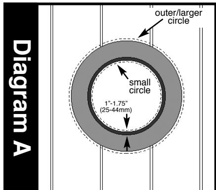
**Step 1.** For 4" (102mm) high flashings, draw a circle 1" (25mm) smaller than the inside of the turret base onto the roof panel. For 6" (152mm) high flashings, draw a circle 1-3/4" (44mm) inside of the turret base. Draw a second line outlining the outer flange perimeter. **Diagram A**
