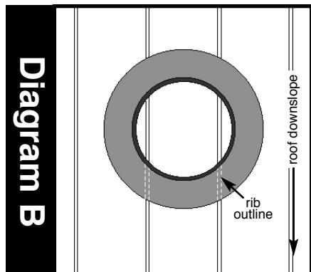
**Step 2.** On the lower half of the flashing, trace the intersecting outline of the roof panel rib(s) onto the base flange and turret section as shown. **Diagram B**
