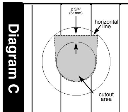
**Step 3.** Remove flashing. For 4" (102mm) high flashings, draw a horizontal line 2" (51mm) above top edge of smaller circle. For 6" (152mm) high flashings, draw a horizontal line 2-3/4" (70mm) above top edge of smaller circle. From the two points where this line intersects the outer circle, connect two straight lines to the small circle as shown. With tin snips, cut roof panel along resulting tulip shaped line (marked cutout area). **Diagram C**
