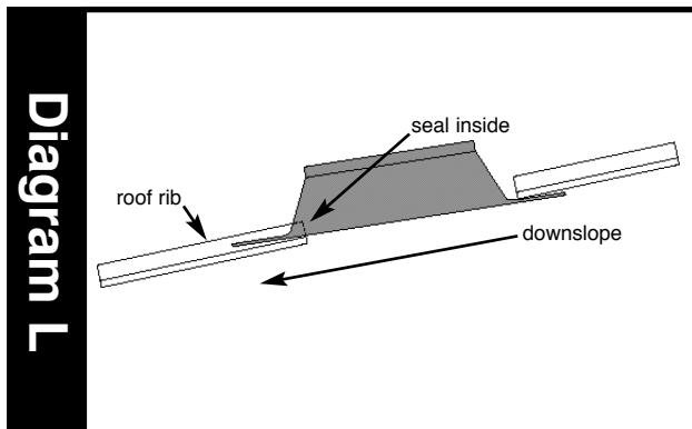
**Step 10.** Force a  $1/2"$  (13mm) bead of polyurethane roof sealant into all exposed overlap joints and fastening penetrations. Force into crevices, then detail and feather edges with putty knife. Be sure to cover all exposed butyl tape with polyurethane sealant as butyl tape is not designed to be exposed to outside elements. This will also prevent dirt and dust buildup on the butyl tape.
